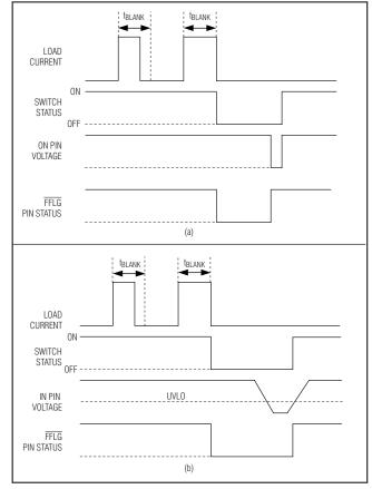
Figure 3. MAX4826/MAX4828/MAX4830 Latch-Off Fault Blanking
